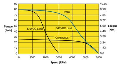
The NeoMetric 922 motor will meet the requirements. RMS torque falls within the continuous duty cycle and total torque vs. velocity falls within the intermittent range.
