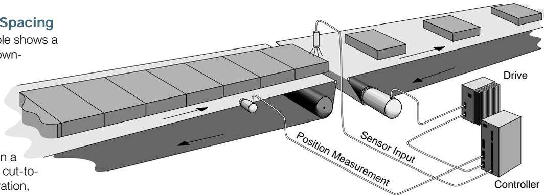
conveyor. The controller waits for the entire product length to leave the master conveyor before it superimposes a distance-shift (i.e., a short fast advance) to introduce uniform product spacing on the slave conveyor. This advances each product a specific distance ahead of the next product as they move onto the second (or following) conveyor.
