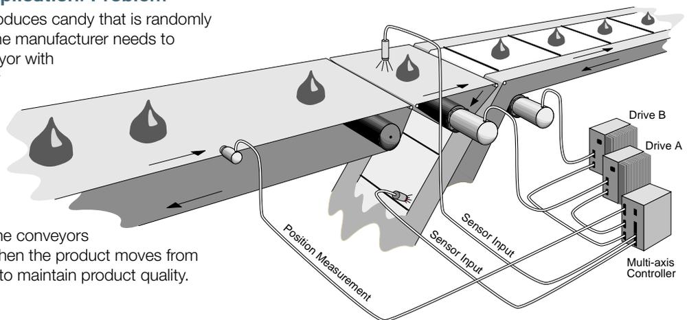
product sensor. Both the correction and exit conveyors are moving, or slaving, at a 1:1 relationship with the infeed conveyor, or master axis. The conveyors are following the feedback from the encoder on the infeed conveyor.
