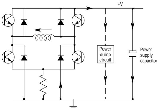
A small increase in supply voltage during regeneration is acceptable, but if the rise is too great the switches may be damaged by over-voltage rather than excessive current. To resolve this problem, we use a power dump circuit that dissipates the regenerated power.
