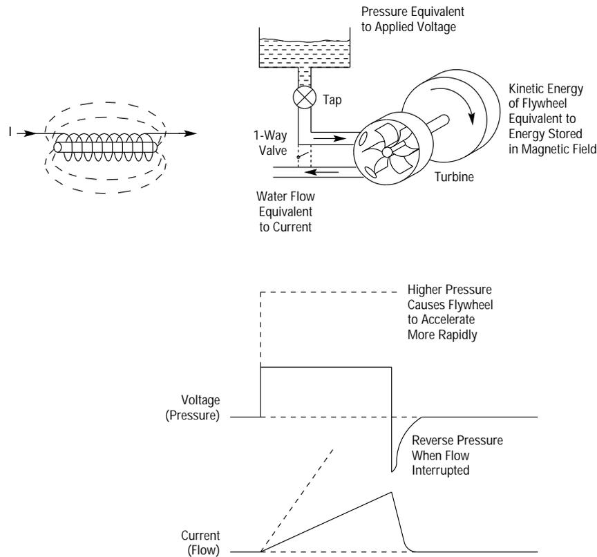
Applying a voltage to the terminals of an inductor produces a similar effect. With a pure inductance (i.e., no resistance), the current will rise in a linear fashion for as long as the voltage is applied. The rate of rise of current depends on the inductance and the applied voltage, so a higher voltage must be applied to get the current to rise more quickly. In a practical inductor possessing resistance, the final current is determined by the resistance and the applied voltage.
