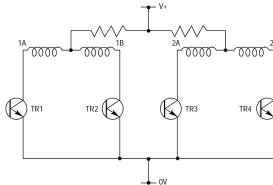
Such a drive will function perfectly well at low stepping rates, but as speed is increased, the torque will fall off rapidly due to the inductance of the windings.
