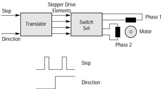
The logic section of the stepper drive is often referred to as the translator. Its function is to translate the step and direction signals into control waveforms for the switch set (see Fig. 2.1). The basic translator functions are common to most drive types, although the translator is necessarily more complex in the case of a microstepping drive. However, the design of the switch set is the prime factor in determining drive performance, so we will look at this in more detail.
