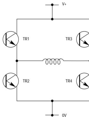
Fig. 2.8 Bipolar R-L drive
