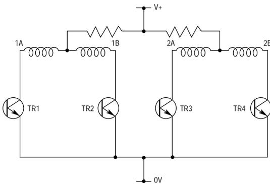
A drawback of the unipolar drive is its inability to utilize all the coils on the motor. At any one time, there will only be current flowing in one half of each winding. If we could utilize both sections at the same time, we could get a 40% increase in amp-turns for the same power dissipation in the motor.
